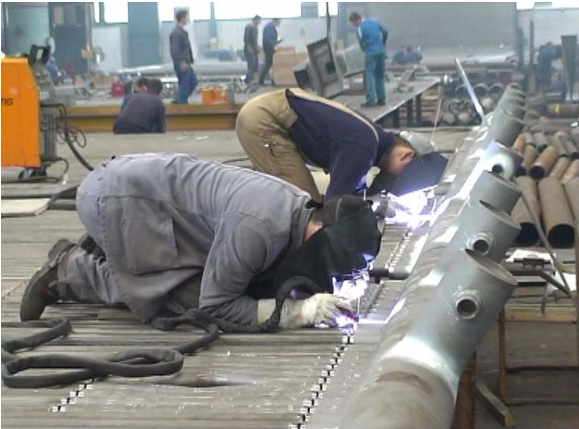
*Figure 3. Manual TIG butt welding of pipes on boiler chamber*
