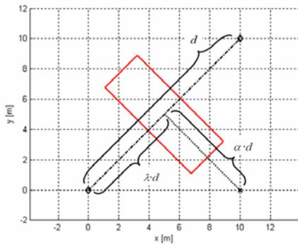
Figure 5: Schematic of the „ghost goal-point“ method of circumnavigating local minima
