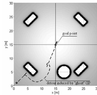
Figure 6: Recreated trajectory planning simulation in a relatively cluttered theater of operation with the local minima avoidance scheme implemented
