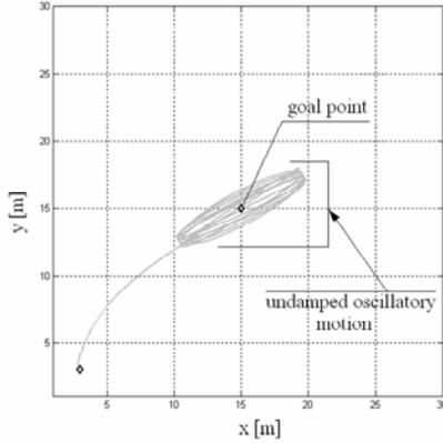
Figure 2: Oscillatory BIBO stability of the algorithm tested with 1 centrally positioned goal-point.
