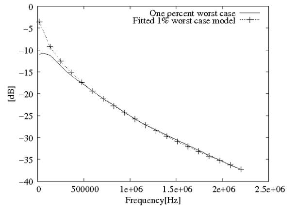
Figure 4 - The 1% worst-case model of the insertion gain
