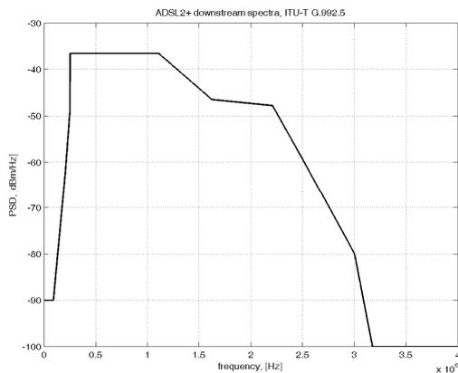
*Figure 8 - ADSL2+ downstream allocated power*
