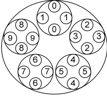
Figure 1 - Basic group cross section and pair numbering
