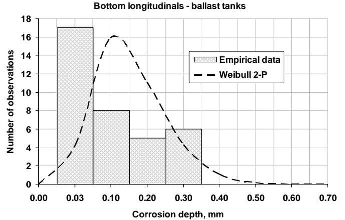
Figure 7. Weibull 2-P probability density function of the corrosion wastage of bottom longitudinals in ballast tanks
