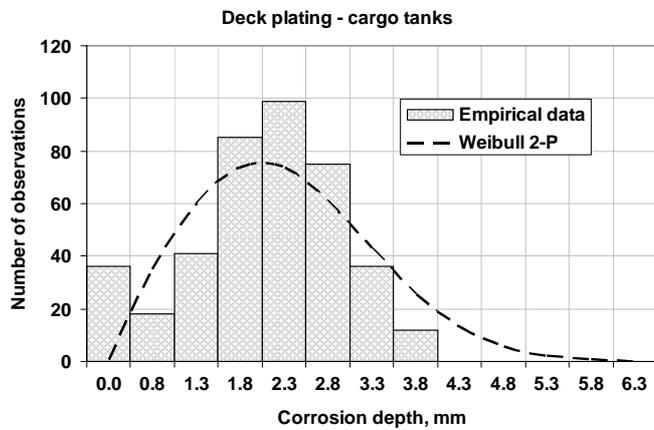
Figure 4. Weibull 2-P probability density function of the corrosion wastage of deck plating in cargo tanks
