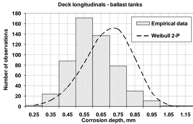
Figure 3. Weibull 2-P probability density function of the corrosion wastage of deck longitudinals in ballast tanks
