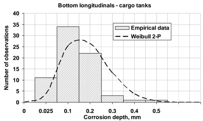
Figure 6. Weibull 2-P probability density function of the corrosion wastage of bottom longitudinals in cargo tanks
