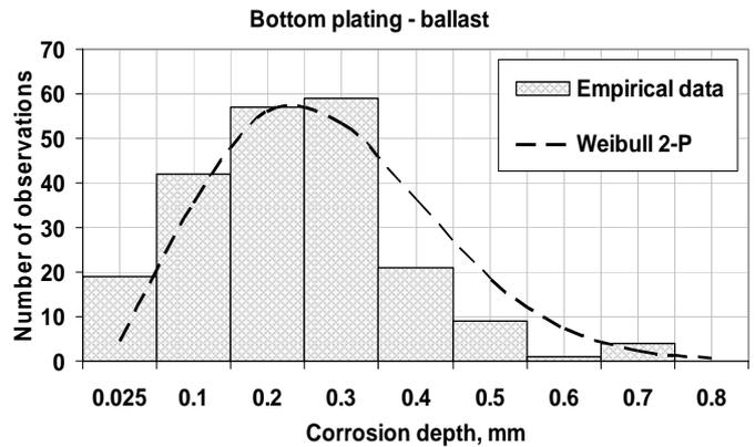
Figure 9. Weibull 2-P probability density function of the corrosion wastage of bottom plating in ballast tanks
