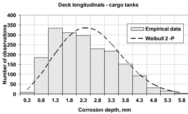
Figure 2. Weibull 2-P probability density function of the corrosion wastage of deck longitudinals in cargo tanks
