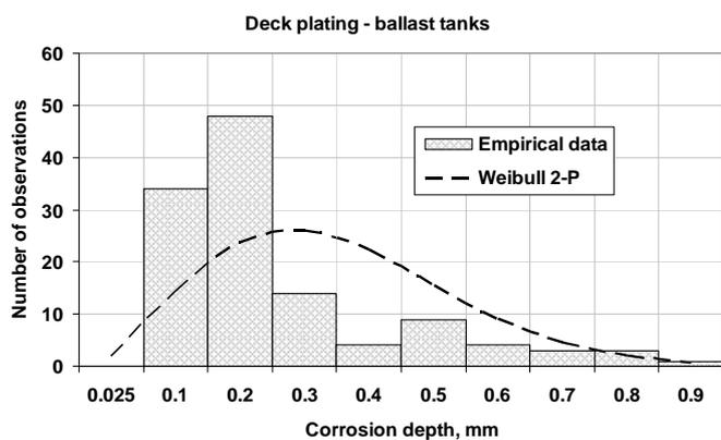
Figure 5. Weibull 2-P probability density function of the corrosion wastage of deck plating in ballast tanks
