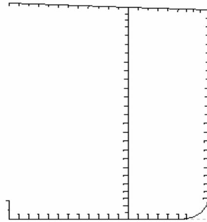
Figure 1. Midship section of single-hull oil tanker in cargo area
