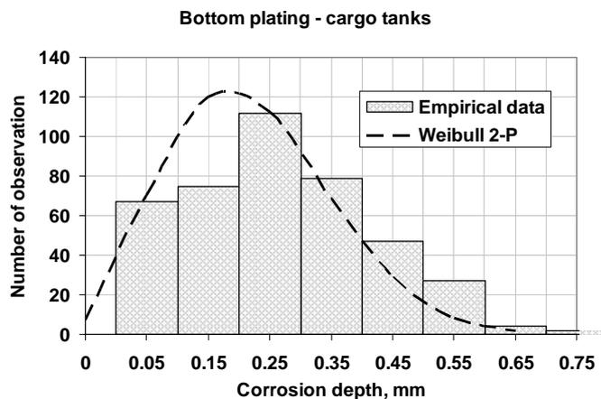
Figure 8. Weibull 2-P probability density function of the corrosion wastage of bottom plating in cargo tanks
