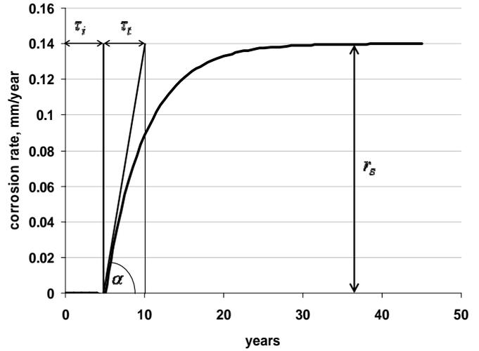
Figure 10. Model of corrosion rate variation with time of the main deck plating in cargo tanks
