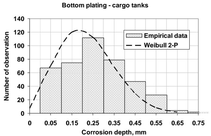
Figure 8. Weibull 2-P probability density function of the corrosion wastage of bottom plating in cargo tanks
