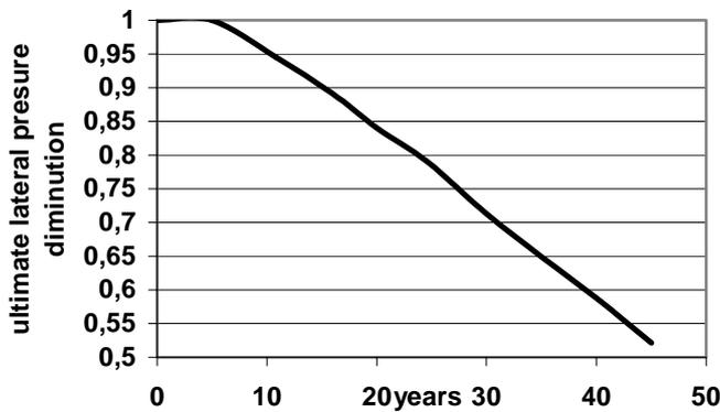
Figure 12. Diminution of the ultimate lateral pressure on the main deck plating in cargo tanks due to local inter-frame bending based on long-term mean corrosion depth variation
