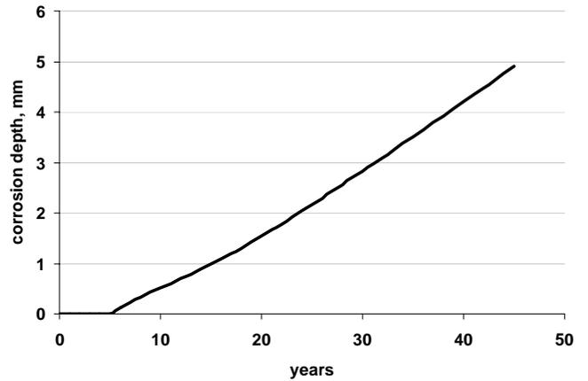
Figure 11. Model of long-term mean corrosion depth variation of the main deck plating in cargo tanks
