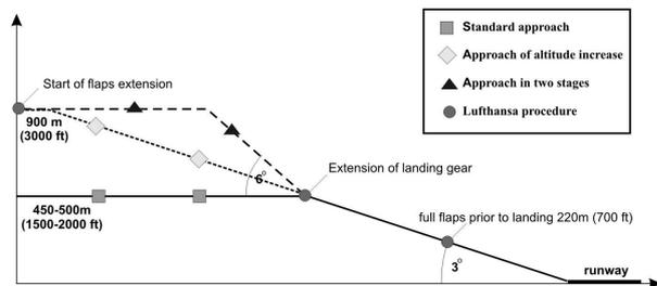
**Figure 2.** Models of landing procedures applicable at Zagreb Airport
