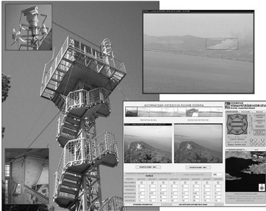
Figure 3. Monitoring unit and user interface of experimental intelligent forest fire monitoring system iForestFire.
