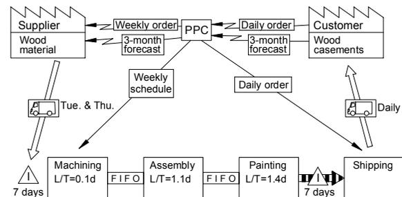
**Figure 1. Material and information flow in the production process**
