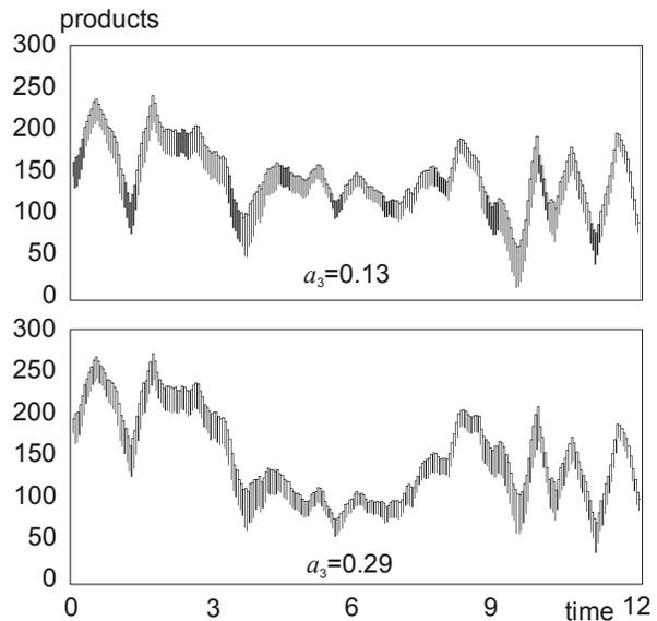
**Figure 12. Inventory level in finished product warehouse for the two different Factor 3 values ( $a_3 = 0.13$  and  $a_3 = 0.29$ )**
