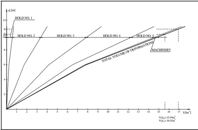
Figure 12. The total volume of local deformations for all holds
