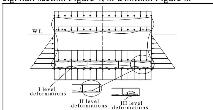
Figure 4. Presentation of transverse local deformation level
