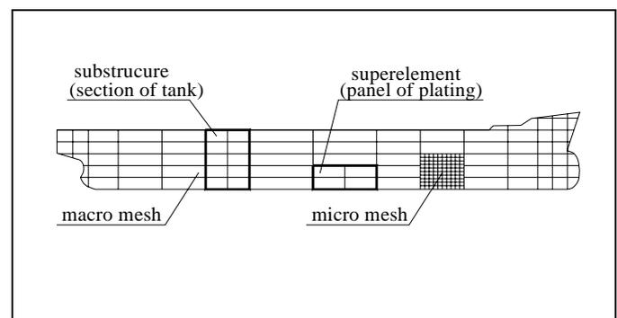
Figure 5. Finite elements mesh of the ship's hull
