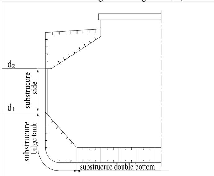
Figure 7. Bulk-carrier hull substructures
