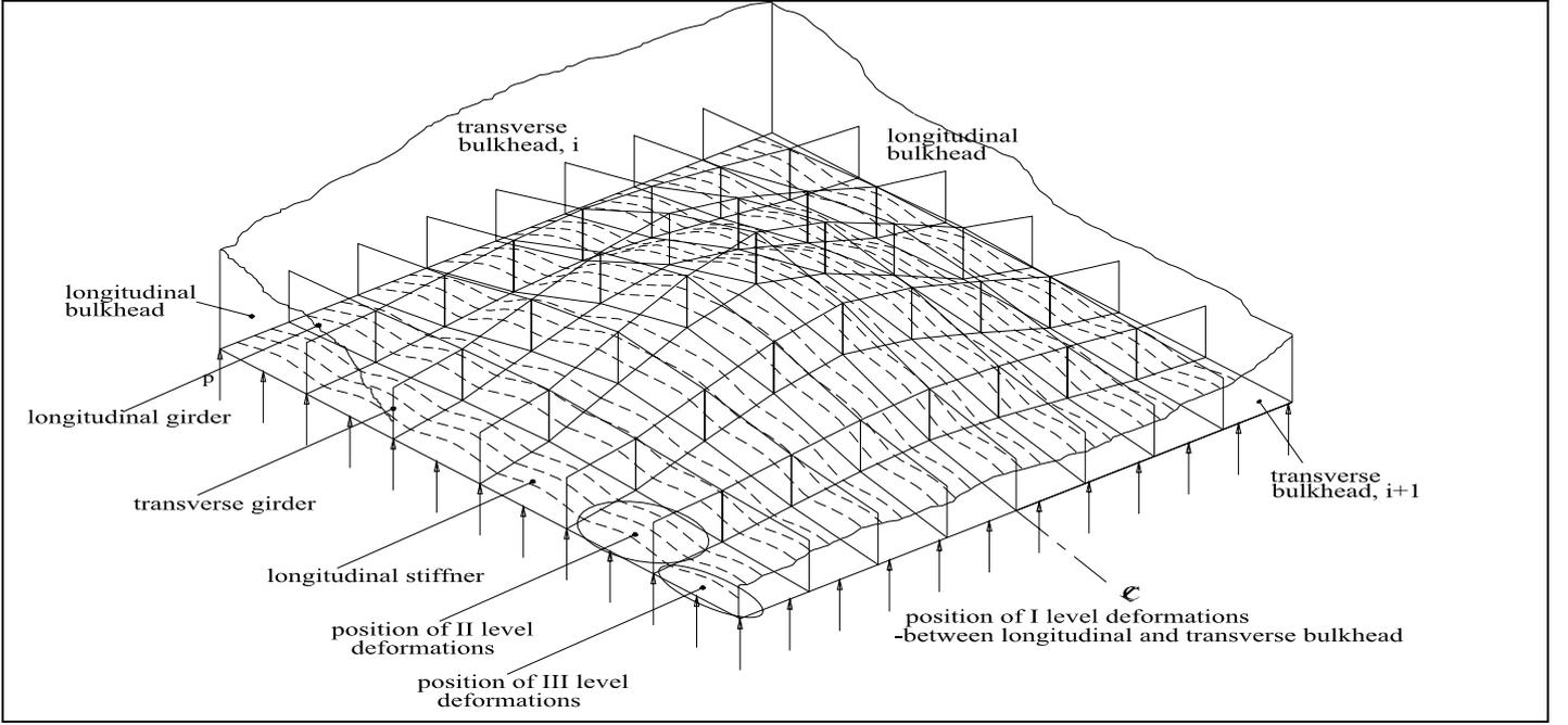
Figure 6. Local deformation levels of ship's bottom
