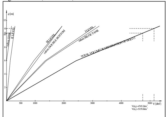
Figure 11. The volumes of local deformations at Hold no. 3
