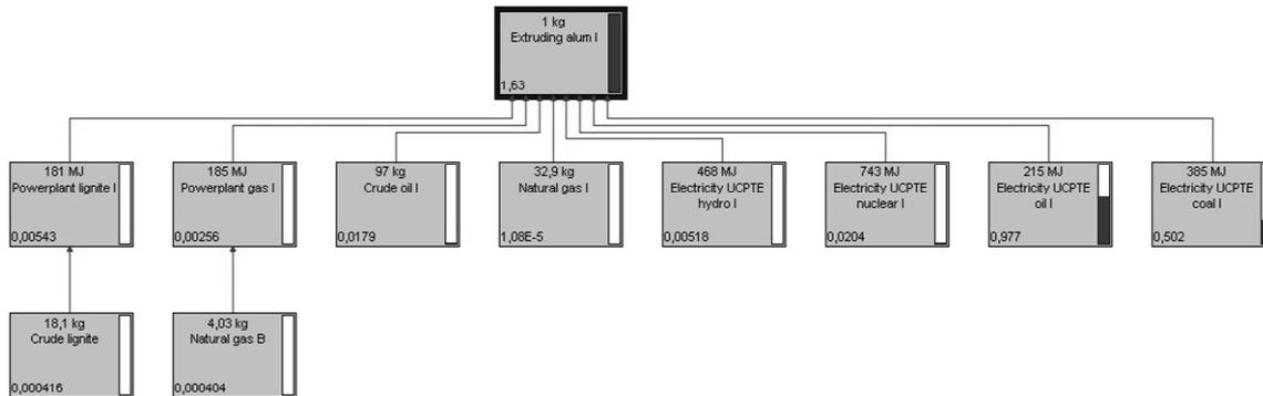
Figure 2 Process tree considered process of tube extrusion [8]
