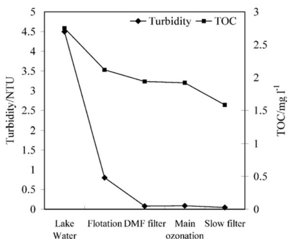
Fig. 2. Turbidity and TOC at different stages of treatment with the conventional trial plant.
