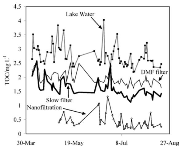
Fig. 7. Comparison of TOC in water treated at a conventional trial plant and in NF permeate when feed water for NF was taken after DMF filtration.
