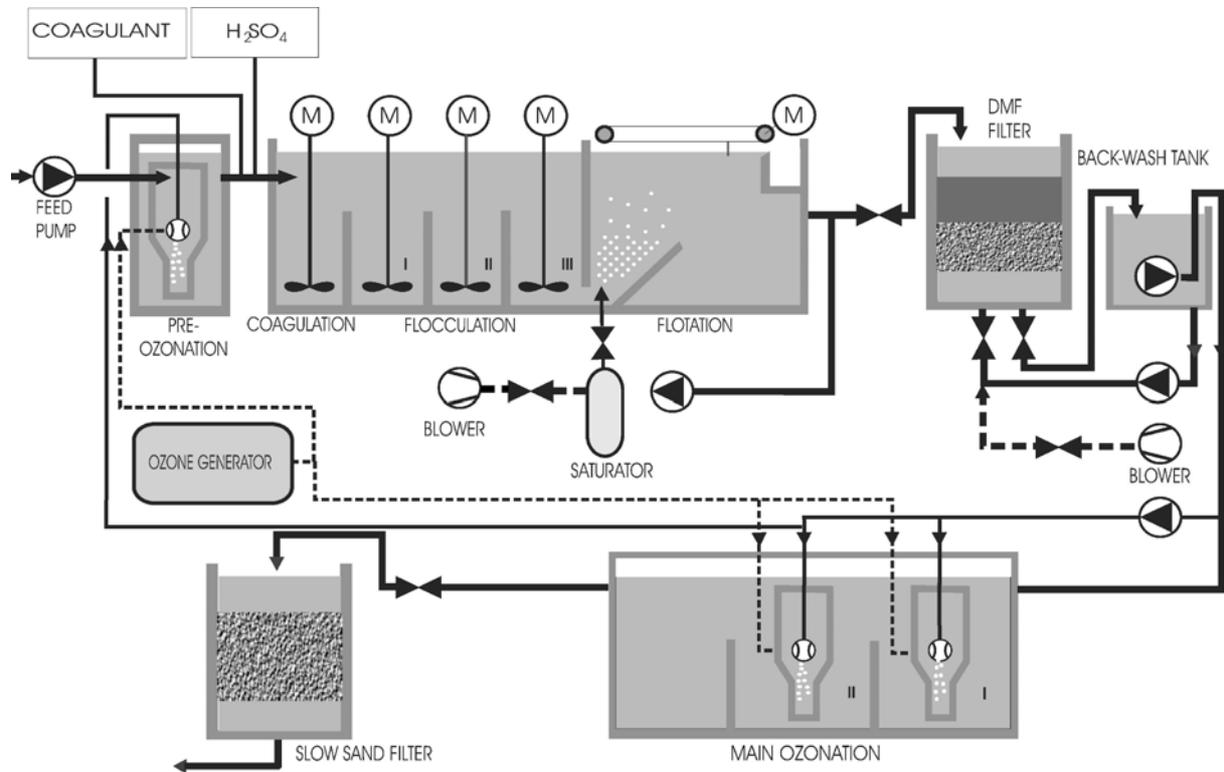
Fig. 1. Scheme of conventional trial plant.
