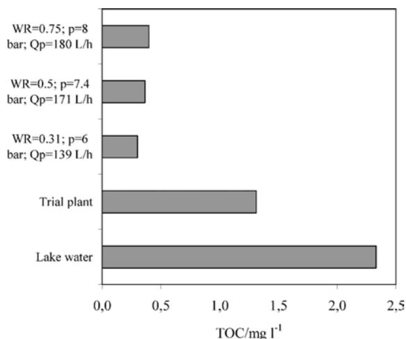
Fig. 5. TOC in lake water, water treated at a conventional trial plant and with a Filmtec NF membrane at different water recoveries (WR) for feed lake water.
