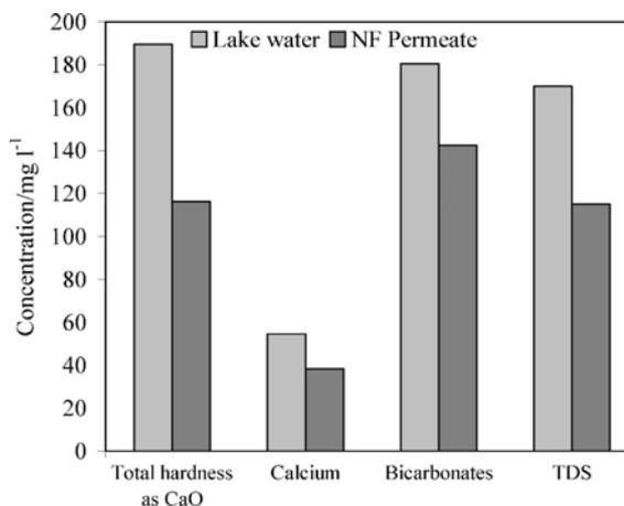
Fig. 6. Concentration of inorganic salts in lake water and NF permeate at  $Y = 0.75$  for feed water taken after DMF filtration.
