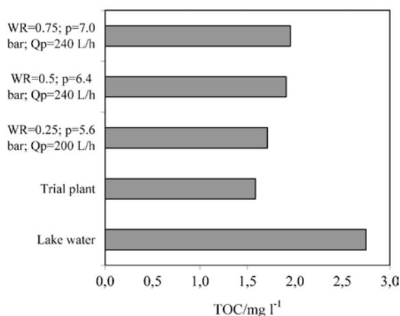
Fig. 4. TOC in lake water, water treated at a conventional trial plant and with the Mavibran UF membrane at different water recoveries (WR).
