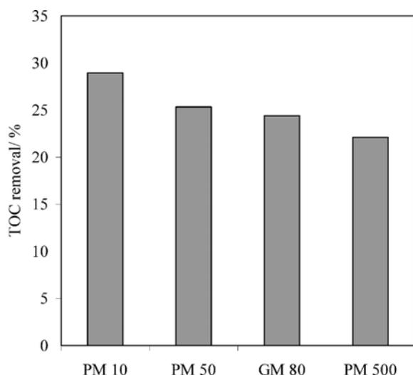
Fig. 3. TOC removal with Romicon hollow-fibre membranes with feed lake water.
