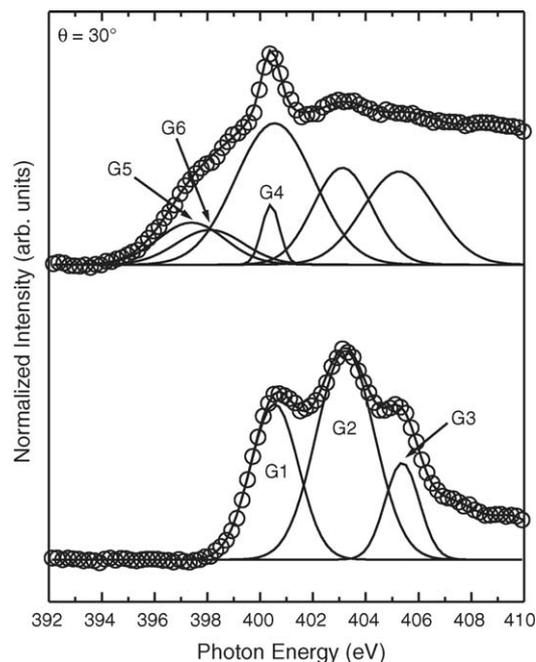
Fig. 3. Normalized N K-edge NEXAFS spectra from as-grown and 2 keV nitrogen ion bombarded p-GaN taken at a photon impact of 30°. The solid lines are a numerical fit of the experimental data (open circles). The introduction of three new resonances G4, G5 and G6 are evident with ion bombardment.
