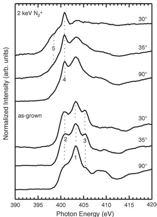
Fig. 2. Polarization dependence of N K-edge NEXAFS spectra of as-grown and 2 keV  $N_2^+$  ion bombarded samples. At the low (grazing) angles of 35° and 30°, features 4 and 5 become more prominent, indicating their  $\pi^*$ -symmetry.
