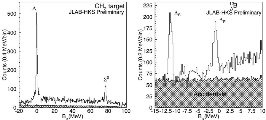
Figure 1. Left: Preliminary spectrum of  $\Lambda$  and  $\Sigma^0$  obtained from the  $p(e,e'K^+)\Lambda(\Sigma^0)$  reaction using a  $\text{CH}_2$  target. Right: Preliminary spectrum of  ${}_{\Lambda}^{12}\text{B}$  hypernuclei obtained from about 90 hours of beam time with current of  $30 \mu\text{A}$ .
