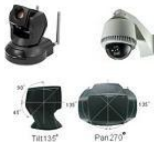
Fig.2. IP camera with Pan, Tilt, Zoom
