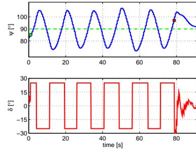
Fig. 1. Charlie's heading and rudder angle during one of the self-oscillation experiments (green circle marks the beginning and red square the end of data recording).
