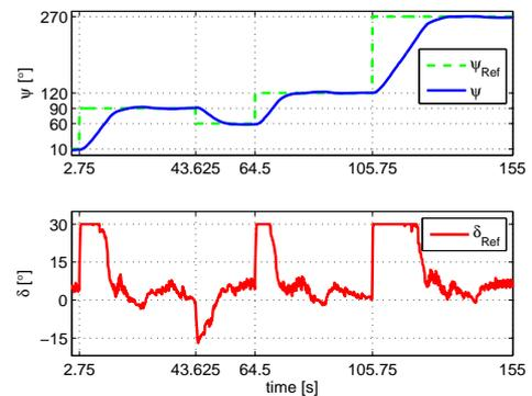
Fig. 3. Heading and rudder angle with the KF controller.
