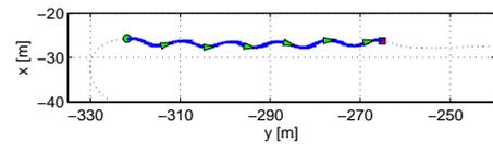
Fig. 2. Charlie's path during one of the self-oscillation experiments (green circle marks the beginning and red square the end of data recording, dotted line is the path before and after the experiment).
