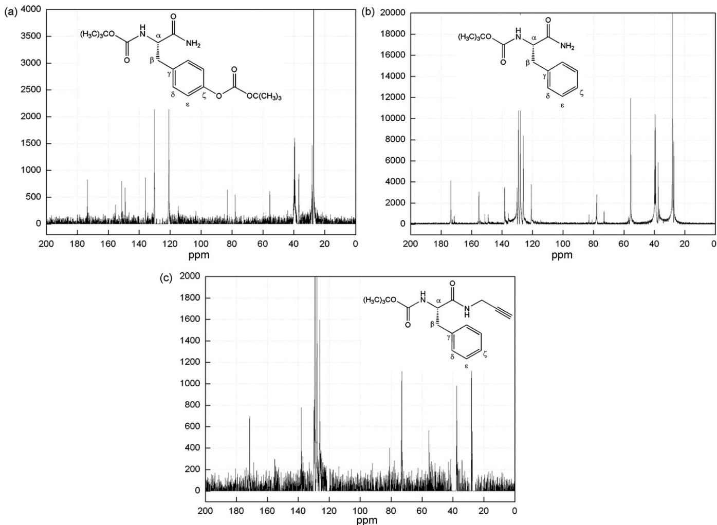
Fig. 6. <sup>13</sup>C NMR magnitude spectra of the estimated pure components: (a) PC<sub>1</sub>; (b) PC<sub>2</sub>; (c) PC<sub>3</sub>.
