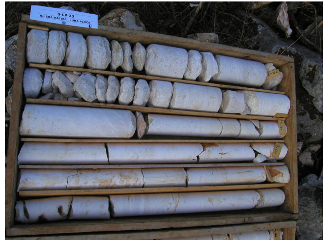
Figure 2. Rock mass core from exploration drilling
