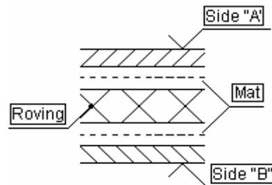
Figure 1. Schematic layout of reinforcement in the matrix of plates
