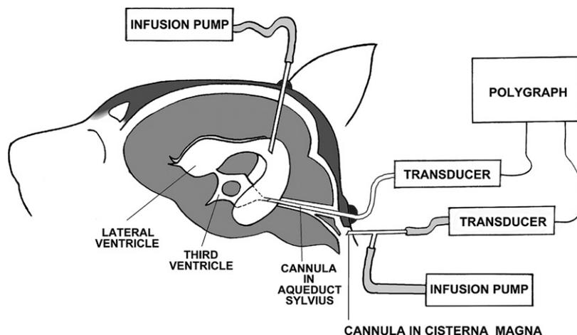
**Fig. 1.** Scheme of an experimental model showing the position of the cannulas for the CSF pressure recording in the aqueduct of Sylvius and the CM, as well as a cannula in the lateral ventricle and “T” connection to the cannula in the CM used for an intraventricular or intracisternal infusion of the mock CSF, respectively.
