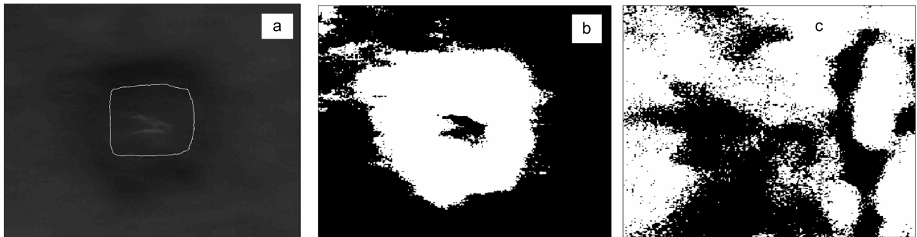
Fig. 5. (a) Demarcation line calculated by applying the level set clustering algorithm on the image shown in Fig. 1a; (b) and (c) spatial maps extracted from fluorescent RGB images shown in Figures 1a and 1c by means of K-means clustering algorithm with interclass distance parameter set to 45.
