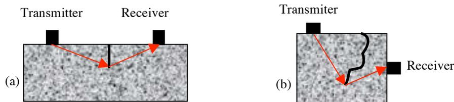
**Figure 13: Crack depth measurement principle (a) non-direct method, (b) semi-direct method.**
