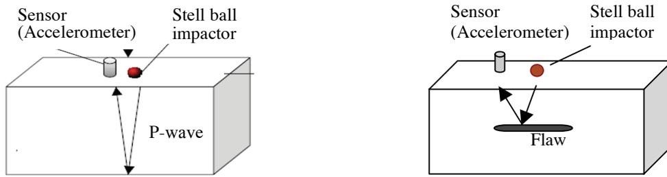
**Figure 3: (a) P-wave reflection from element boundary (b) P-wave reflection from flaw.**
