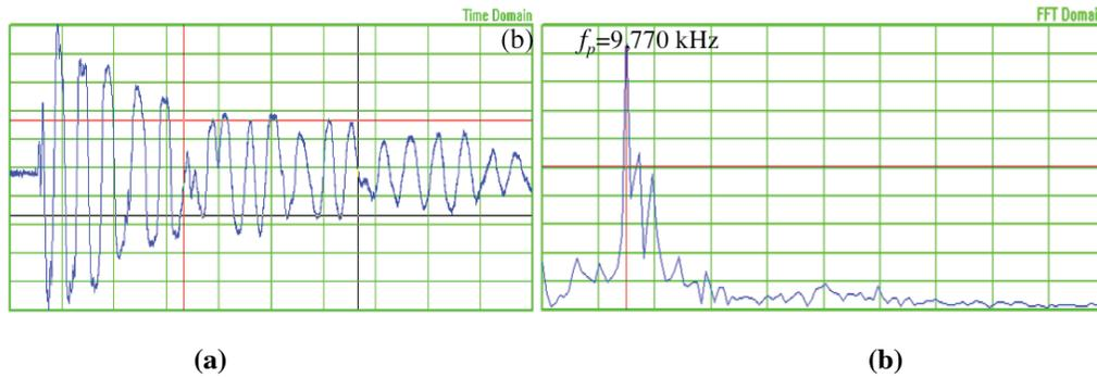
**Figure 4: (a) Measured data in time domain, (b) Measured data in frequency domain after  $FFT$ .**
