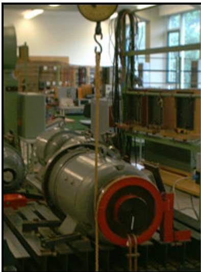
Figure 9. Parallel DC laboratory motor 3 kW [1].
