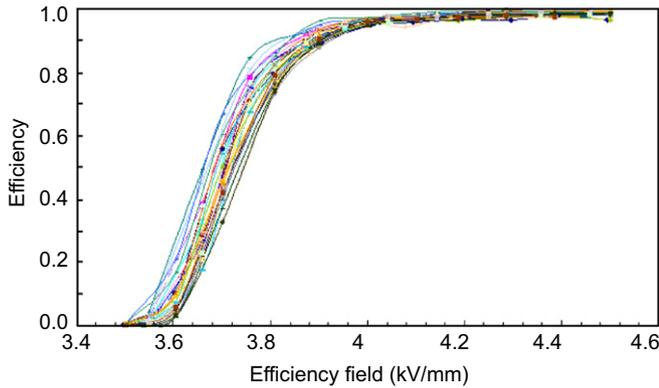
Fig. 2. Efficiency as a function of the nominal electric field  $E_0 = V_0/g$ , for 32 GRPCs. All the chambers show a similar behaviour reaching the full efficiency for  $E > 4.0$  kV/mm. Ar/C<sub>2</sub>H<sub>2</sub>F<sub>4</sub>/Iso – C<sub>4</sub>H<sub>10</sub>/SF<sub>6</sub> = 48/47/4/1%.
