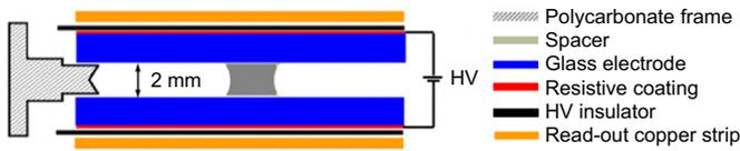
Fig. 1. Schematic drawing of a Glass Resistive Plate Chamber.
