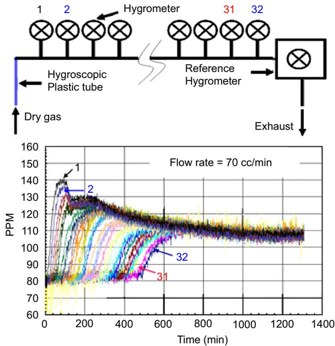
Fig. 6. Top: Experimental setup used for the calibration. Bottom: response of the 32 hygrometers after the insertion of 10 cm plastic tube inside a stainless steel line.
