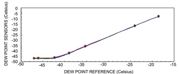
Fig. 5. Calibration curves for all the 32 Honeywell HiH-4602-C sensors with respect to the MTS5(GE Panametrics) hygrometer ( $\equiv$  reference).
