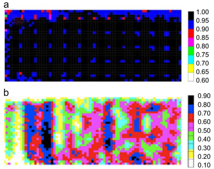
Fig. 3. (a) Efficiency map of a single GRPC at  $E_0 = 4.4$  kV/mm. The spacer dead area determines the lower efficiency in correspondence of their location. (b) efficiency map at 3.75 kV/mm: as the efficiency strongly depends on the gap value, the effect of local variation of the distance between the electrodes is clearly visible. Ar/C<sub>2</sub>H<sub>2</sub>F<sub>4</sub>/Iso – C<sub>4</sub>H<sub>10</sub>/SF<sub>6</sub> = 48/47/4/1%.
