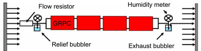
Fig. 4. Gas distribution in the VETO system (see text).
