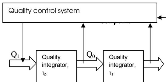
Fig.3. A two-step quality control system
