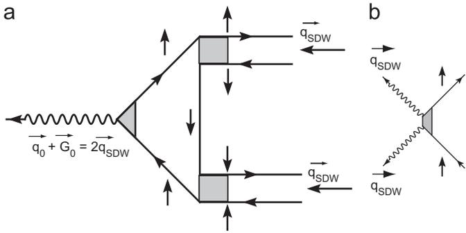
**Fig. 2.** Umklapp coupling of two SDWs enhanced at  $\vec{q}_{SDW}$  (a) to intracell charge fluctuations and/or to phonons linearly coupled to carriers and (b) to phonons coupled quadratically to the carriers. Internal structure of the electronic triangle is governed by the  $A_g, B_g$  symmetry properties of the outgoing vertices and by the  $U_d$  or  $\tilde{U}$  nature of the incoming square vertices which flip the spins.
