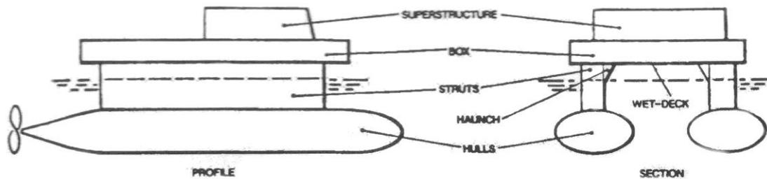
**Figure 4:** Main Features of a SWATH vessel
