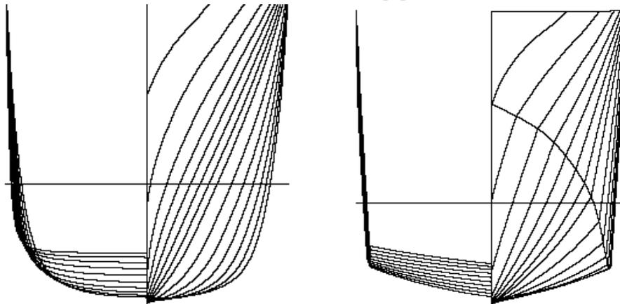
**Figure 2:** Round Bilge (left) and Hard Chine (right) Hull Shapes of Catamarans
