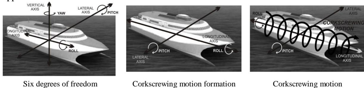
**Figure 7:** Formation of corkscrewing motion
