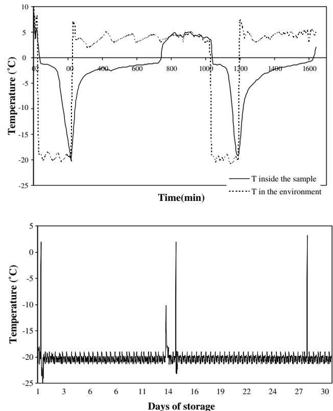
Fig. 4. Temperature and time profile during two cycles freezing and thawing of sea bass fillets ( $T$  freezing:  $20 \pm 2$  °C;  $T$  thawing:  $+4 \pm 1$  °C) (a). Temperature of the freezer during 30 days of frozen storage (b).
