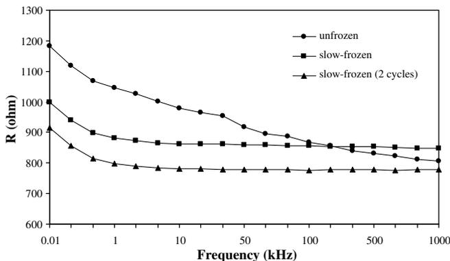
Fig. 1. Resistance spectra of sea bass samples – preliminary experiment.
