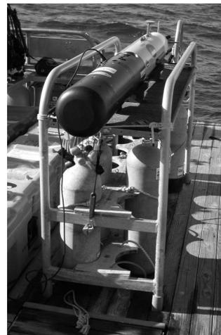
Fig. 1. The Hydroid Remus vehicle.
