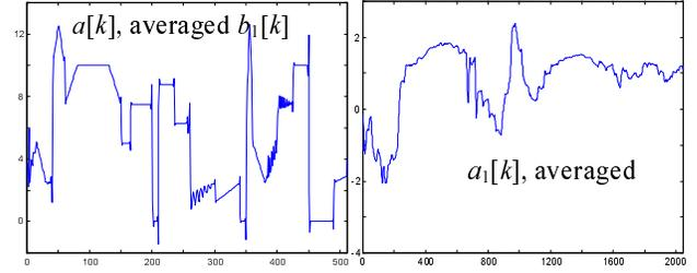
**Figure 13.** Left: Approximation coefficients from example in **Figure 10** computed by averaged filter parameters  $b_1[k]$ . Right: averaged filter parameters  $a_1[k]$  from **Figure 11**
