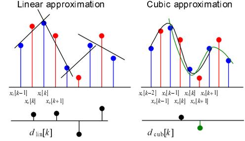
Figure 4. Modified scheme. Approximation polynomials do not necessarily contain known points. They are rather set to minimize some property of the signal  $d[k]$  (e.g., the energy of  $d$  in some neighborhood of the observed step  $k$ ).
