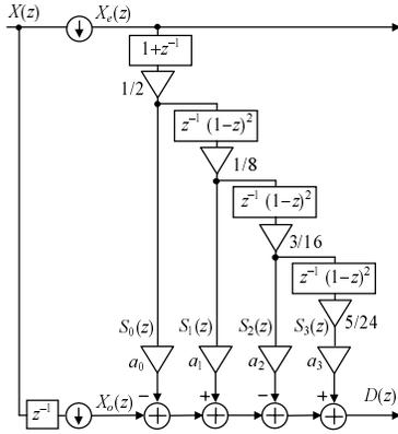
Figure 3. Realization of the lifting step.
