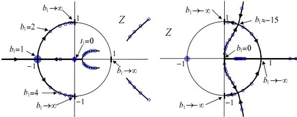
**Figure 7.** Zero locus plots of the LP filter, parameter  $b_1$ .
