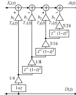
Figure 5. Realization of the dual lifting step
