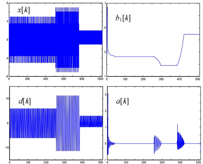
**Figure 9.** Top left: analyzed signal  $x[k]$  composed from 3 sine waves ( $\omega = 9\pi/12, 10\pi/12, 8\pi/12$ ). Top right: filter parameter  $b_1[k]$  adapted by the least squares algorithm on interval  $[k-20, k+20]$ . Bottom left: detail  $d[k]$ . Bottom right: residual approximation coefficients  $a[k]$ .
