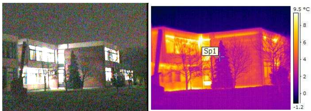
Illustration 7: Characteristic thermal bridges on the corners of a building
