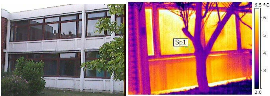
Illustration 6: Linear thermal bridge on ground floor and wall connection
