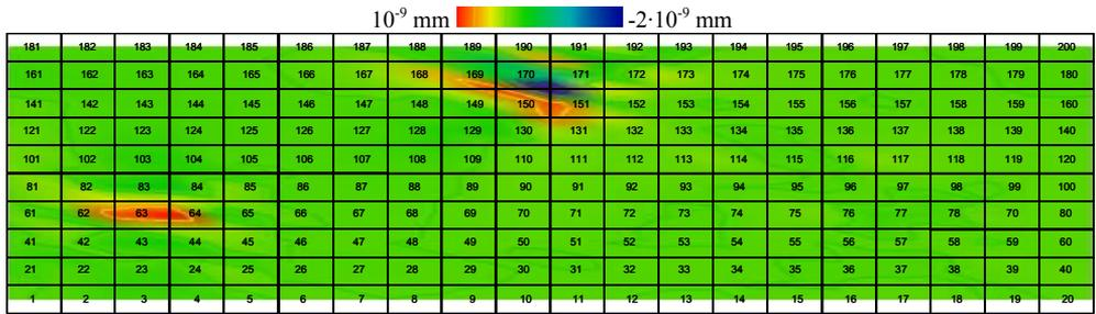
Figure 8: Curvature difference in direction y for measurement point 1
