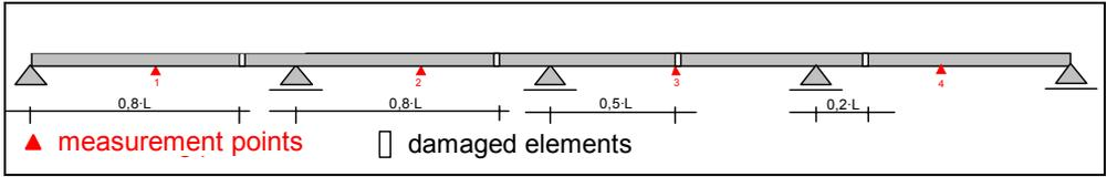
Figure 1: Damaged model: reduction of bending stiffness in finite elements 40, 90, 126, 160
