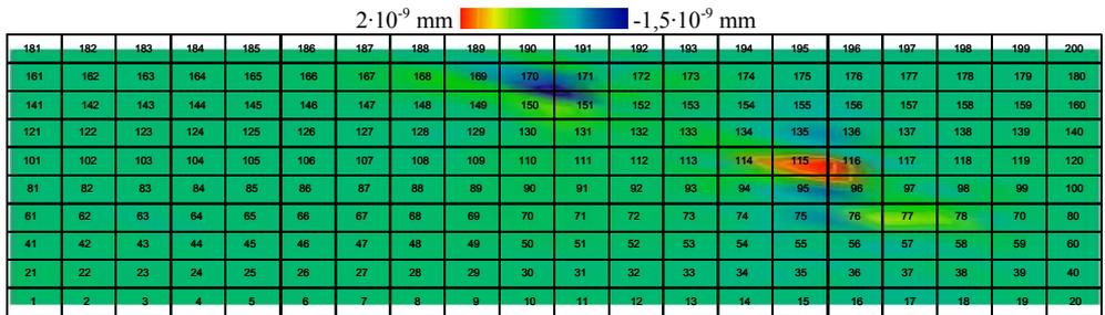
Figure 10: Curvature difference in direction y for measurement point 2
