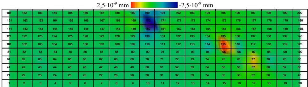
Figure 9: Curvature difference in direction x for measurement point 2
