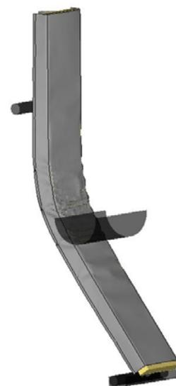
Fig. 3: Bending at the approach angle of 20°, test and numerical simulation
