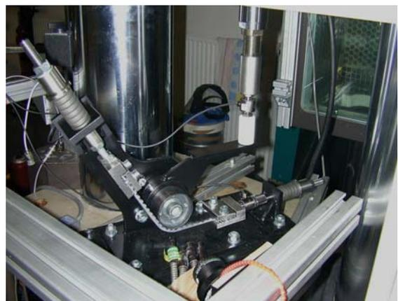
**Fig. 2:** Test set-up for the belt tooth tests.
