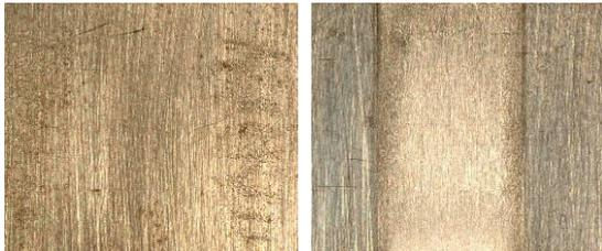
**Fig. 2:** Surface morphology after 2000 shots of polyamide compounds: non-filled (left); 50w% glass fiber (right).
