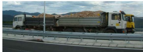
Fig. 3: Dabar Bridge – static loading.
