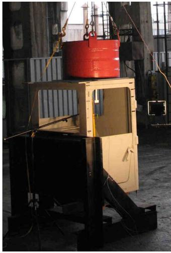
Fig. 4: Experiment - view of the cabin with the loading bob
