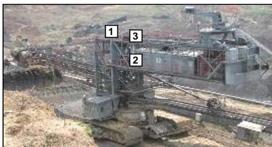
Fig. 1. Selected measuring locations: measuring spot 1 Lamellae of bucket wheel boom; measuring spot 2 – Lower carrier of counter weight structure; measuring spot 3 – Upper carrier of counter weight structure
