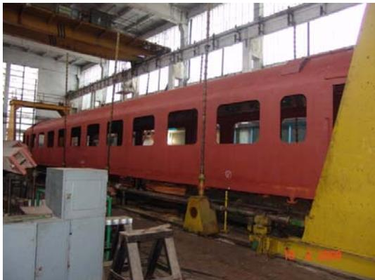
**Fig. 1:** The coach on Stress Analysis Bench Test
