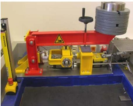
**Fig. 5:** Linear tribometer AMB
