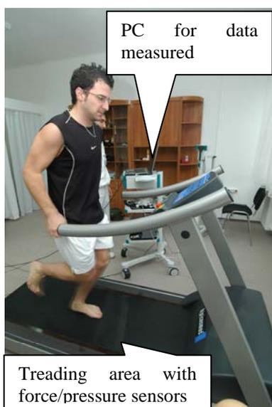
**Fig. 1:** Instruments of simplified gait analysis
