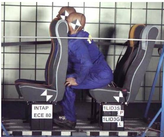
**Fig. 1:** Impact of a head to a head restraint during vehicle crash test.
