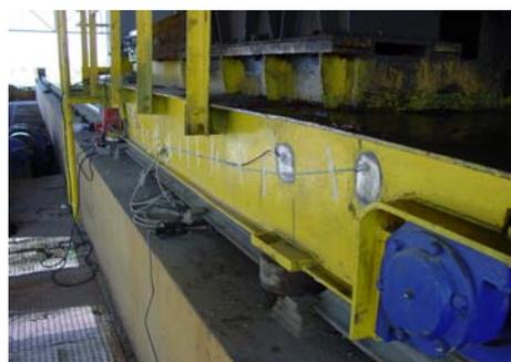
Fig. 2. Measuring system - strain gauges fixed to trolley structure
