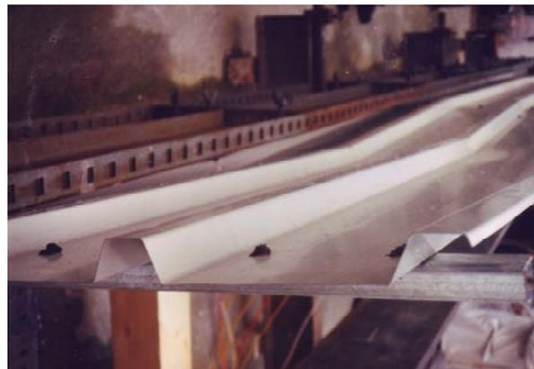
Fig. 7: Trapezoidal Sheet 2 in first span after testing
