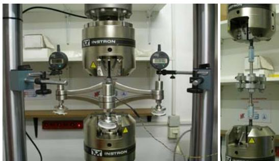
**Figure 1 Axial loading of pairs of spider fittings and spherical joint attachments**
