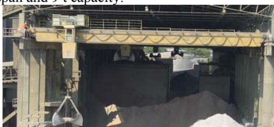
Fig. 1. The bridge crane - 30 m bridge, 9 t capacity
