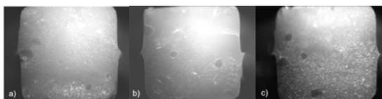
**Fig. 2:** Fracture surfaces of the bone cements prepared by mixing technique powder to liquid.
