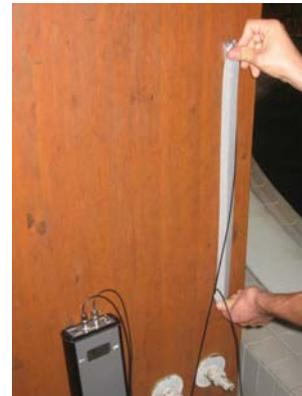
**Fig. 3:** Velocity determination in a lamella
