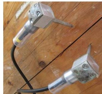
**Fig. 2:** Crack depth determination by acoustics (stress wave sensors)
