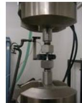
**Fig. 2:** Specimen on the left side and special gripping system used in the HCF tests.
