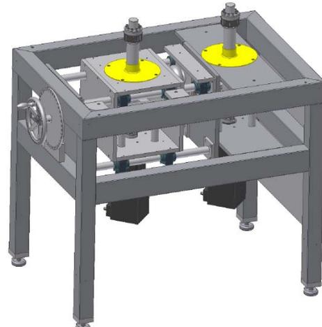
**Fig. 6:** The loading unit with the NCTE (Non-Contact-Torque-Engineering) device integrated.
