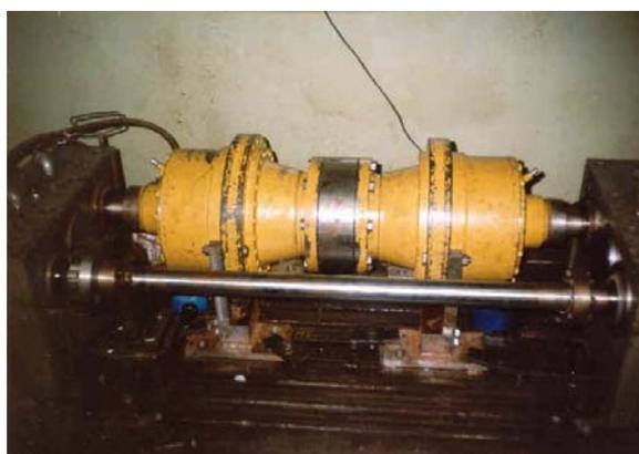
Fig. 2: Testing of planetary gear drives in the back to back system (power circulation)
