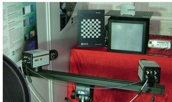
**Fig. 4** Experimental setup with High Speed cameras, calibration target, loudspeaker and frequency generator for vibration measurements.
