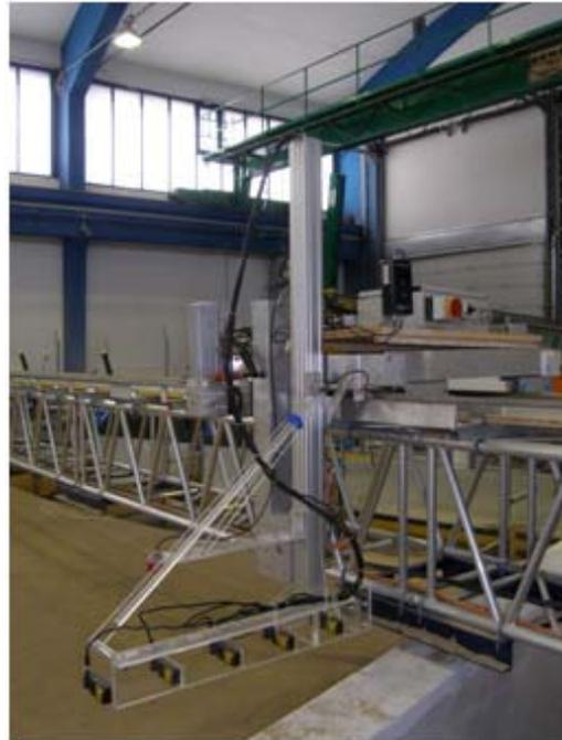
**Fig. 2:** Measuring bridge with the measuring platform and five mounted laser triangulation sensors
