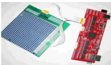
**Fig. 3:** Plantograf V08 – Sensor Matrix with Electronic Circuits
