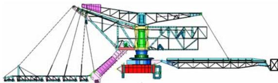
Fig. 5: FEM model of load-carrying structure of excavator
