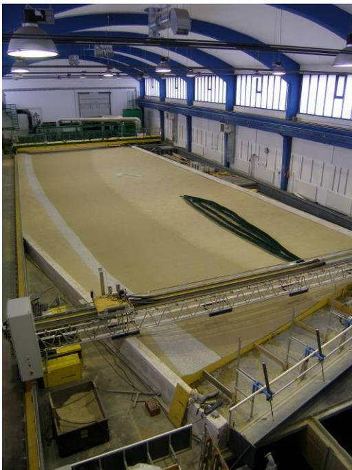
**Fig. 1:** Total view of the model of the Danube to the east of Vienna
