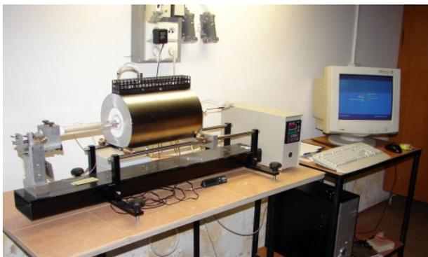
**Fig. 1:** Thermal dilatometer for measuring of volume changes of ceramic material.
