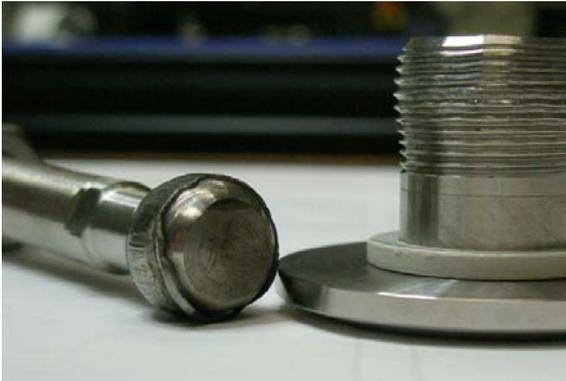
**Figure 4 Yielding of the spherical joint due to the Hertzian stresses and deformation of cylindrical body**
