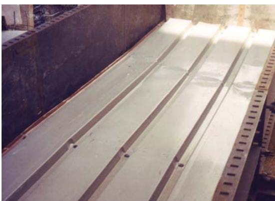
Fig. 6: Trapezoidal Sheet 1 after testing.
