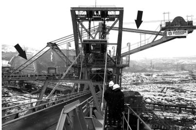
**Fig. 1:** Self-propelled transporter – bands that demand the tension identification marked with arrows.
