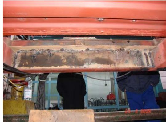
Fig. 6: Longitudinal beam (after reinforcing)
