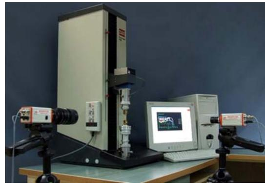
Fig. 1. MTS Synergie 100 loading system and videextensometer system.
