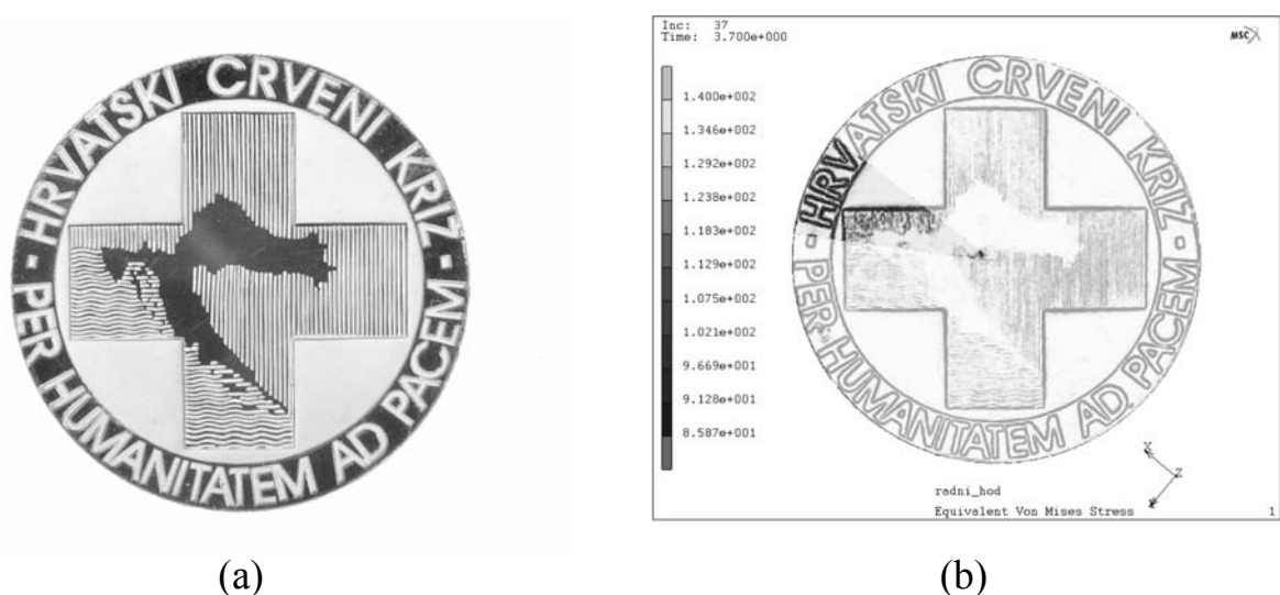
Fig. 1. Red cross medal, (a) Photograph of the obverse, (b) Digitized medal using Atos ® with 1/12 th marked where FE simulation was performed (Courtesy of Damir Mataušić Academic sculptor & medallier)
