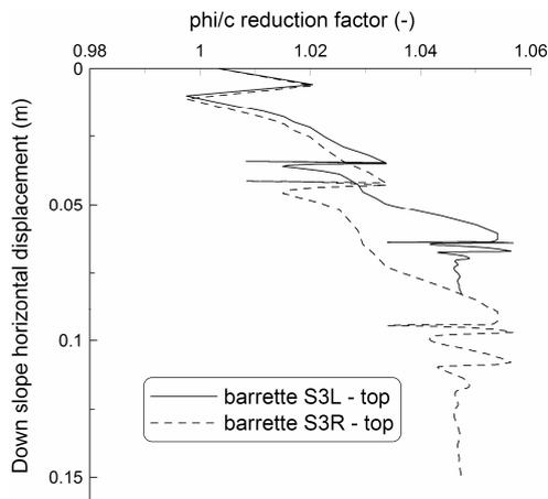
Figure 8. Phi-c reduction analyses with embedded barrettes
