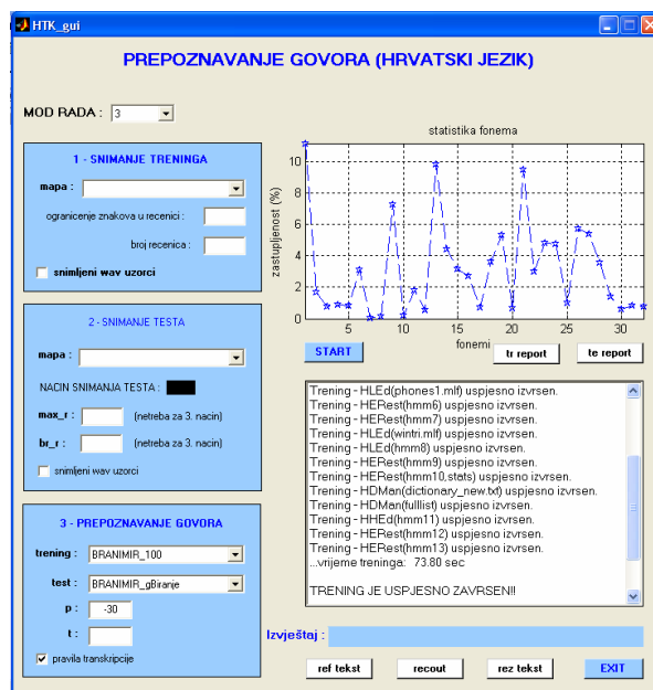
Fig. 2. GUI interface in Matlab for HTK for Croatian language
