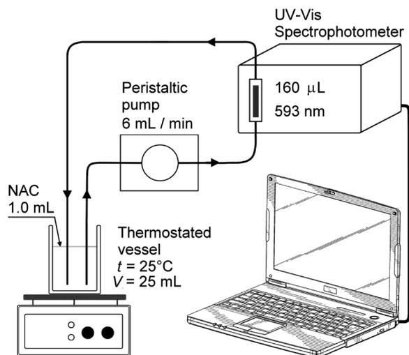
Fig. 1 Kinetic manifold for the spectrophotometric determination of NAC.
