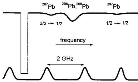
**Fig. 2.** Measured absorption spectrum recorded by scanning the laser across the  $6p^2\ ^3P_0 \rightarrow 6p^2\ ^3P_1$  transition (upper trace) with frequency dispersion marks of the Fabry-Perot interferometer (lower trace). For the  $^{207}\text{Pb}$  lines the values  $F \rightarrow F'$  are indicated.
