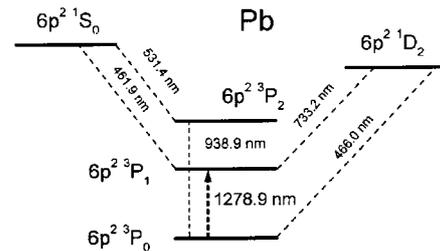
**Fig. 1.** Partial term diagram displaying the ground  $6p^2$  configuration of neutral lead with multipole transitions indicated.
