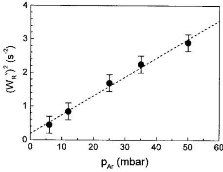
**Fig. 3.** The dependence of the square of the equivalent width of the lead resonance line on the argon pressure. The dashed line represents the least square fit through the measured data.
