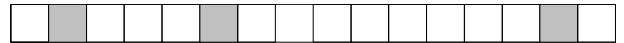
Fig 1. An example of a Bloom filter bit array with m=16 and k=3 with one element added to the set. Grey squares represent bits set to one.
