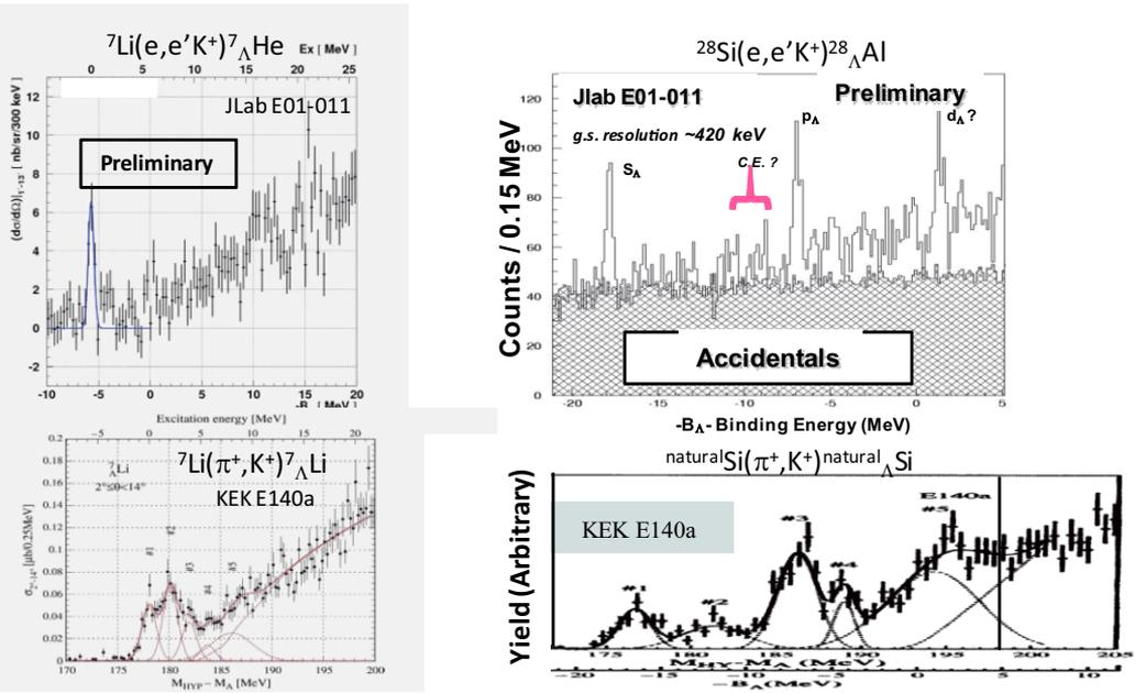
Figure 2: Preliminary hypernuclear mass spectra of the  ${}^7\text{Li}(e, e'K^+){}^7_\Lambda\text{He}$  and  ${}^{28}\text{Si}(e, e'K^+){}^{28}_\Lambda\text{Al}$  reactions with the electron beam at 1.8 GeV. Those of the  $(\pi^+, K^+)$  reaction are also shown below the corresponding spectra.
