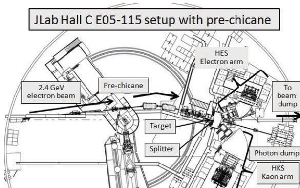
Figure 3: Hypernuclear Spectrometer system in JLab Hall C for E05-115 and the pre-chicane system.
