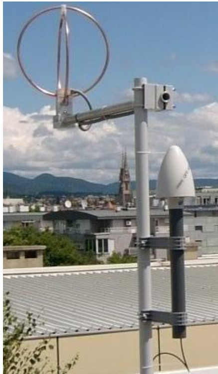
Figure 3 LINET sensor antennas (orthogonal rings) and GPS antenna
