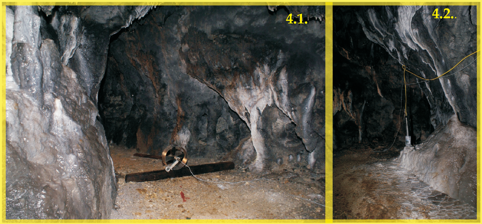
Fig. 4. Monitoring of the wind speed (4.1.), temperature and water chemistry parameters (4.2.)
