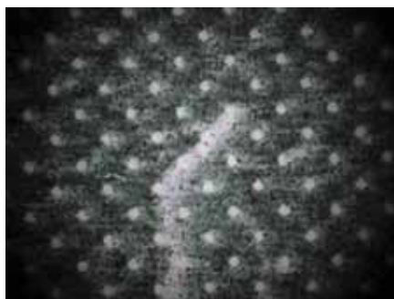
Figure 1. Microscopic images of printing plate and print damages for edition EN br.1,1 (uncoated paper)
