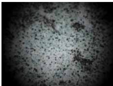
Figure 2. Microscopic images of printing plate and print damages for edition GL br.1,1 (coated paper)
