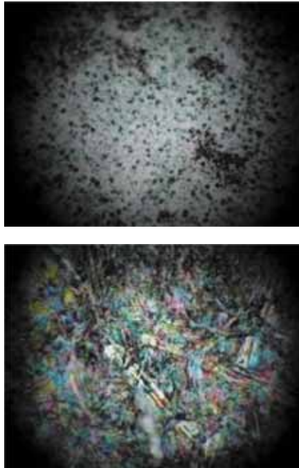
Figure 1. Microscopic images of printing plate and print damages for edition EN br.1,1 (uncoated paper)
