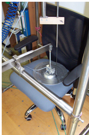
Figure 2. The position of the chair sample, seat loading pad with load-cell and inductive depth meter
