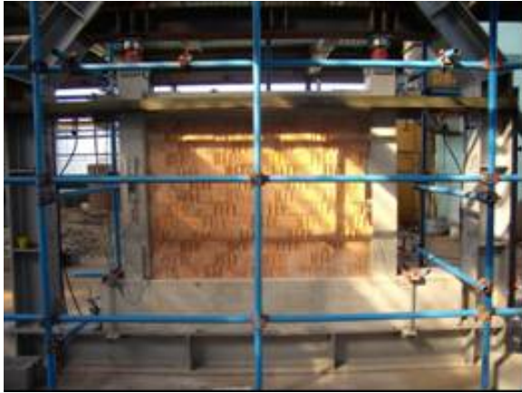
Figure 3. R/C frames infilled with Opeka and Eurotherm hollow clay blocks
