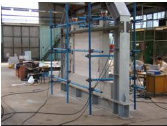
Figure 4. R/C frame infilled with Ytong blocks and Reference bare frame
