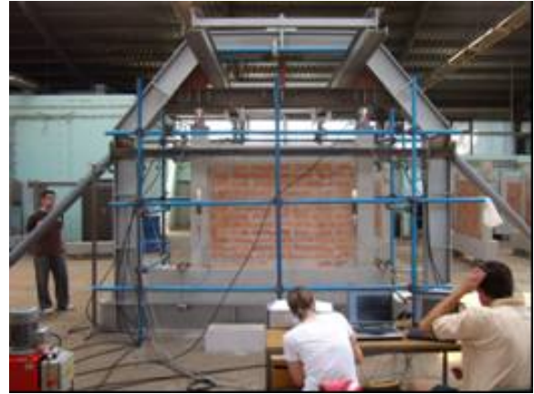
Figure 3. R/C frames infilled with Opeka and Eurotherm hollow clay blocks
