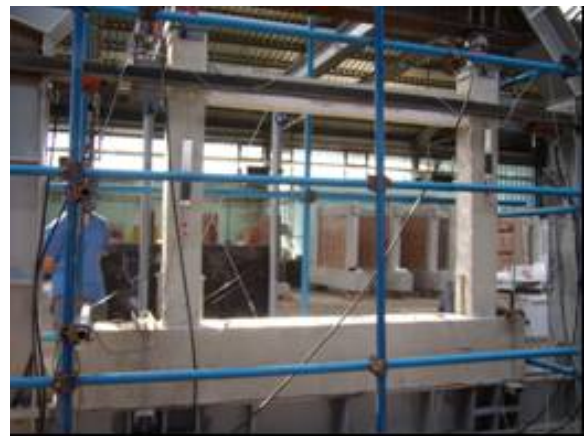
Figure 4. R/C frame infilled with Ytong blocks and Reference bare frame
