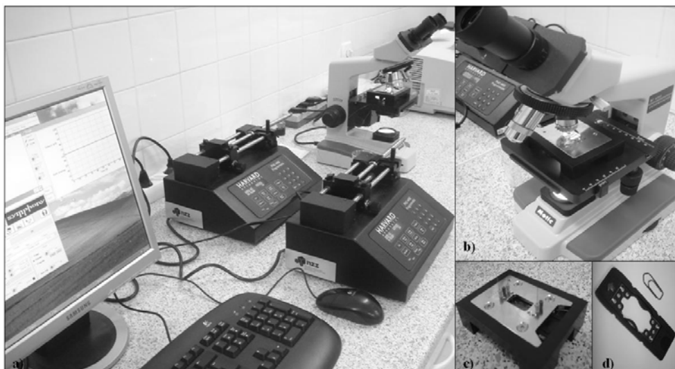
Figure 1: Experimental set up used to perform hexanol oxidation in microreactor. Snapshot of:
