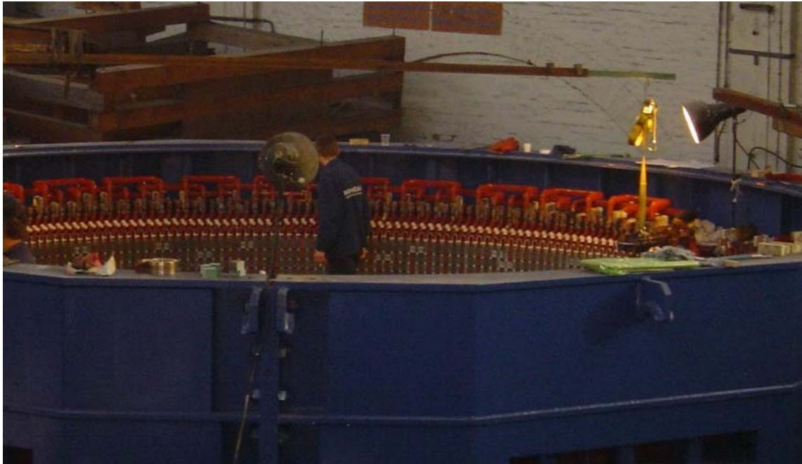
Fig. 4 Insertion of wedges in the generator factory
