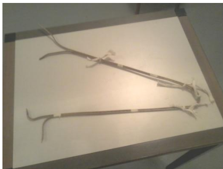
Fig. 5. Part of insulated conductor of the stator winding
