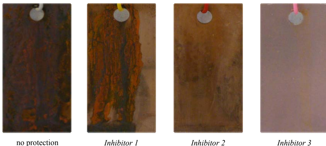
Figure 10. Bronze panels after 336 hours in humidity chamber at 35 °C
