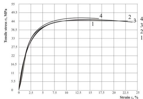
Fig. 1. Diagram tensile stress – strain with the same energy density
