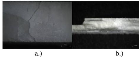
Fig. 6. Brittle fracture of material: a) test specimens of 0.1 mm thickness, b) test specimens of 0.2 mm thickness
