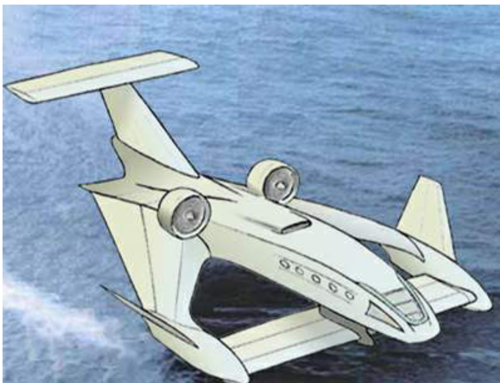
Figure 8. « BRACERA II» - vehicle for transport of 20 passengers, idea project D. Marasović, Bc.S. from Split (speed about 120 knots, EKRANOPLAN)
