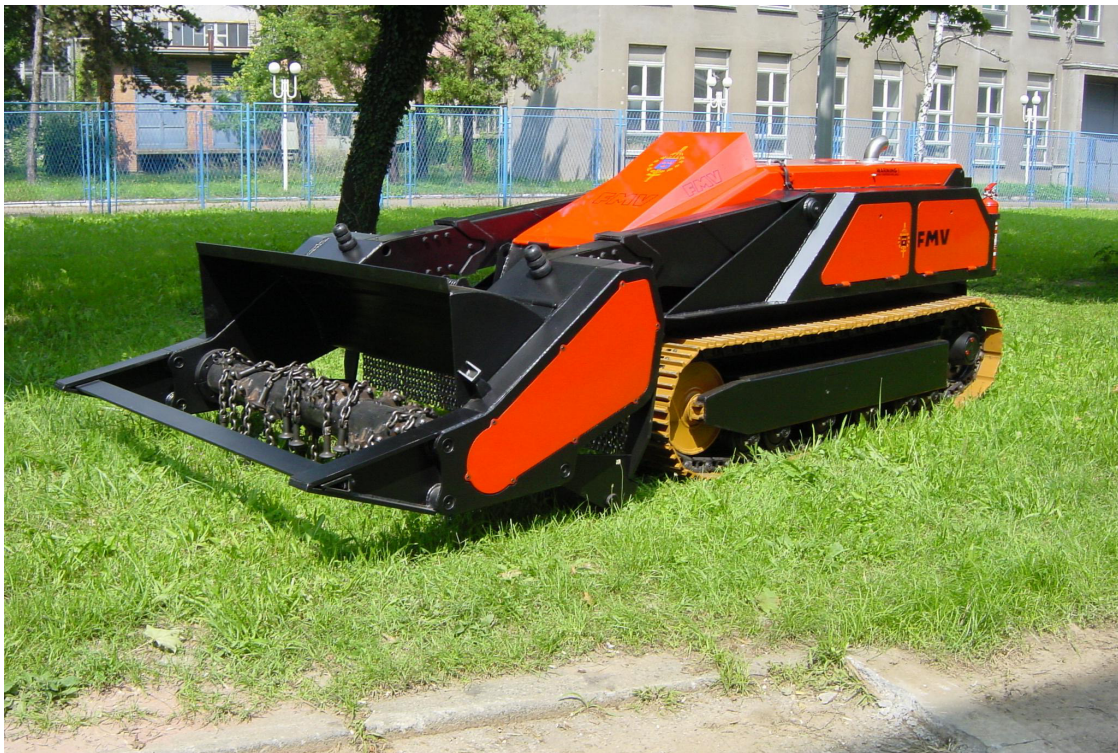
Figure 1. The humanitarian minecleaning machine / Demining machine MV-5
