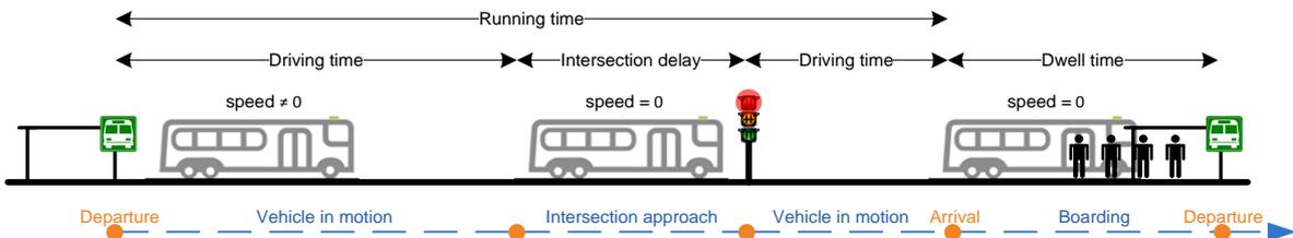
**Figure 1. Different segments of the operation time**
