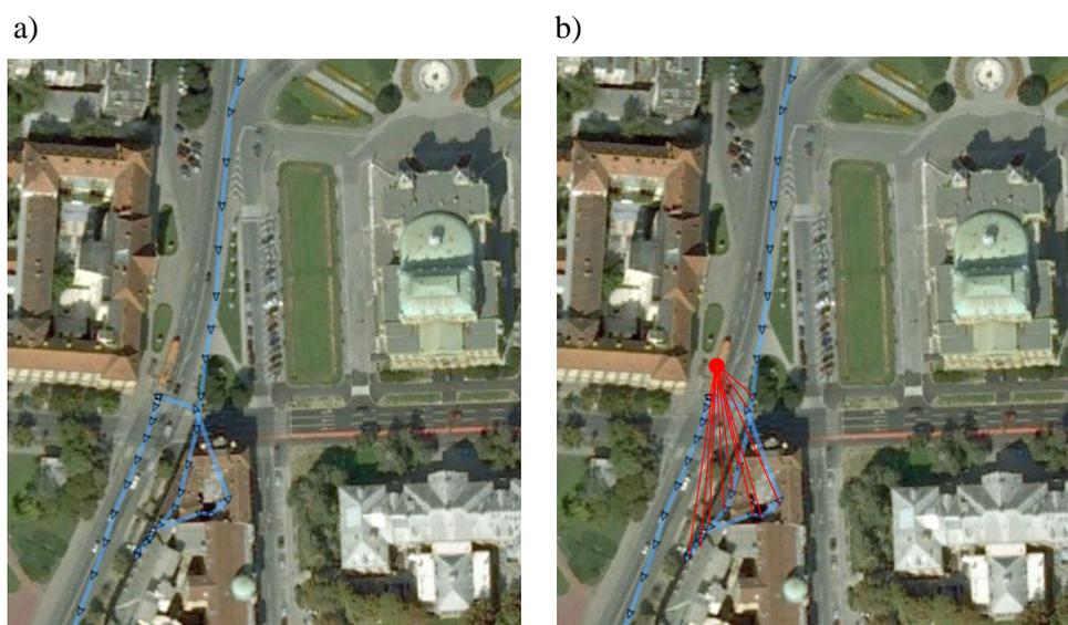
**Figure 2. Recorded GPS track (a) and actual PT vehicle position (b)**
